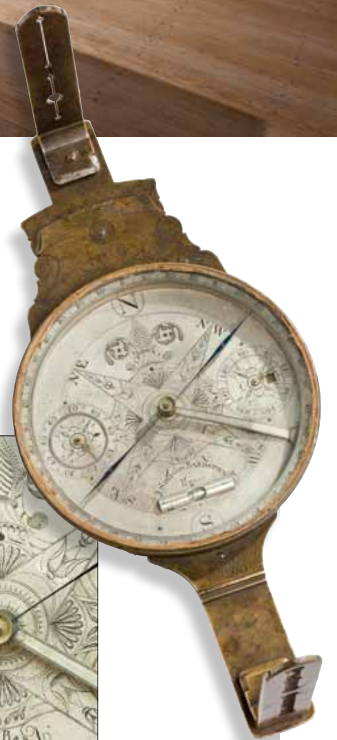
Fig. 12. Detail of a surveyor’s compass made by Jonathan Simpson (1797–1863), Bardstown, Kentucky, 1819. Brass, steel, silver, glass, wood, iron; length 14 ¾, width 6 ⅝ inches. This beautifully engraved compass was originally owned by James Kerr McGoodwin (1793–1875).
